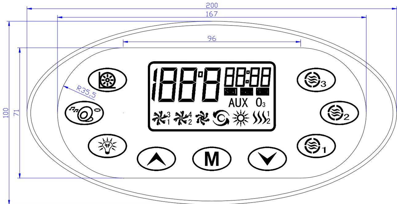
Fig. 2.The installation plan of 9 buttons (200\*100mm)
